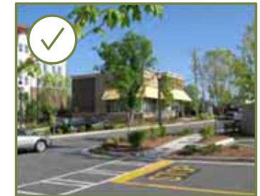
> Example of a commercial street that has adequate sidewalks, crosswalks, ramping, etc.
