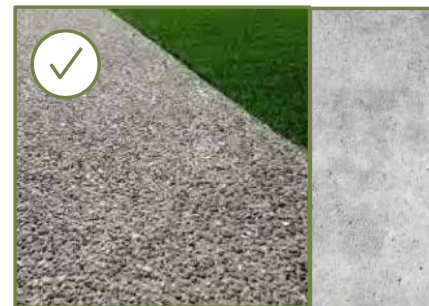
> Exposed aggregate concrete and smooth concrete
